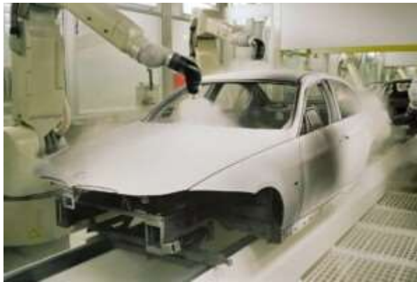
Figure 361: Robot spray painting a car (not Toyota) (Image BMW Werk Leipzig under the CC-BY-SA 2.0 Germany license)
