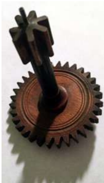
Figure 113: Wooden gear milled by Eli Terry (Image TomVaughn under the CC-BY-SA 4.0 license)
