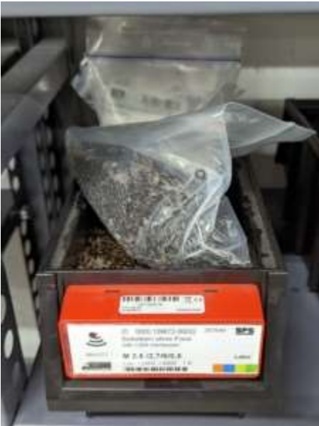
Figure 161: VMI Screws Overfilling (Image Roser)
