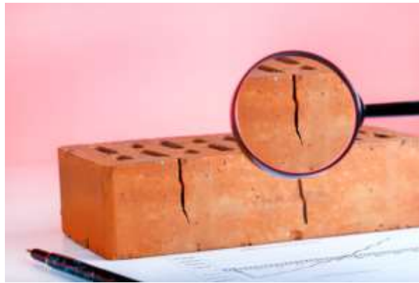
Figure 209: Defective Brick (Image Sergey Chuyko with permission)
