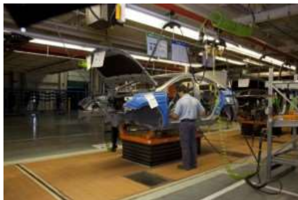
Figure 32: Hyundai moving walkable platform assembly line (Image Carol M. Highsmith in public domain)
