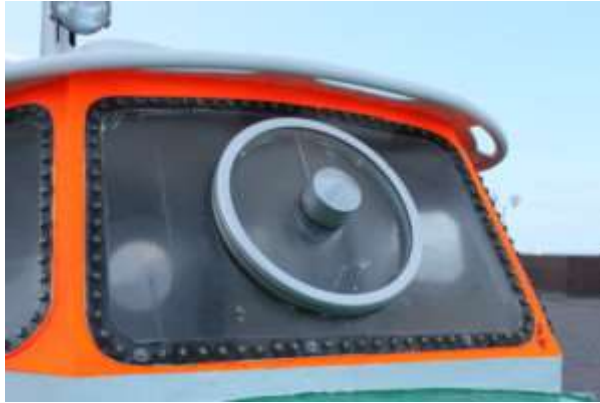
Figure 376: Clear view screen on a boat (Image Bin im Garten under the CC-BY-SA 3.0 license)
