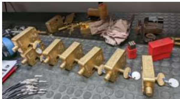
Figure 405: SNCF Railroad locks in service (Image Roser)
