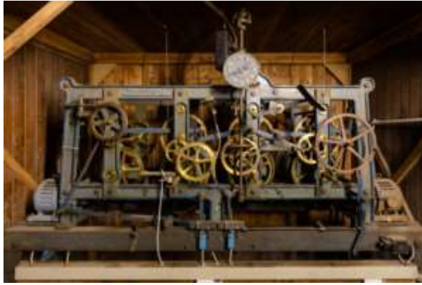
Figure 112: A mechanical metal church clock (Image Dietmar Rabich under the CC-BY-SA 4.0 license)
