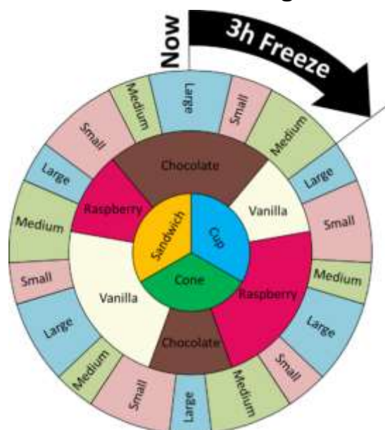
Figure 83: Changeover Wheel Production Freeze (Image Roser)
