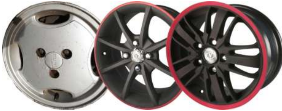
Figure 27: Wheels with 3, 4, and 5 lug nuts (Image Bindydad123 under the CC-BY-SA 4.0 license, and (Image PXHere in public domain)
