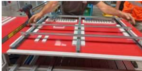
Figure 407: Jigs for assembling switch boxes (Image Roser)
