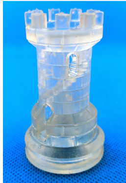
Figure 22: 3D printed tower with internal staircase. (Image Roser)
