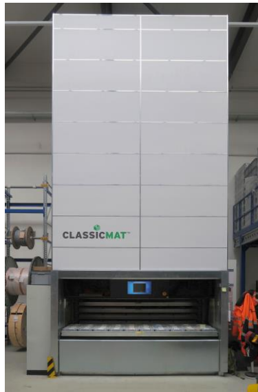
Figure 87: Vertical Lift Storage Example (Image Kecko SBB - EIZ Erstfeld under the CC-BY-SA 2.0 license)
