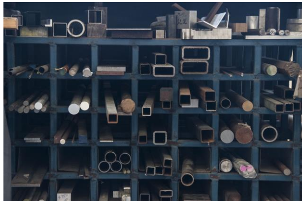
Figure 114: Metal Profile Storage Shelf (Image Tech. Sgt. Ave I. Young in public domain)
