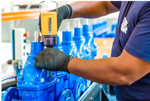
Figure 263: Industrial Valve Manufacturing And Assembly Factory (Image The Light Writer 33 with permission)
