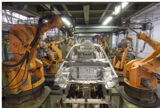
Figure 258: Kuka Industrial Robots assembling car bodies. Image by Mixabest from Wikipedia and available under the CC-BY-SA License (Image Mixabest under the CC-BY-SA 3.0 license)
