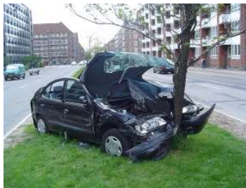
Figure 104: Notice how little the passenger cabin is damaged? (Image Thue in public domain)
