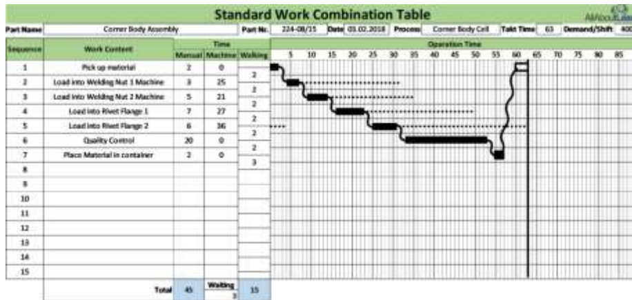
Figure 238: Toyota Standard Work combination example (Image Roser)
