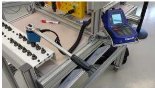
Figure 201: SCANIA Screws Torque Measure (Image Roser)
