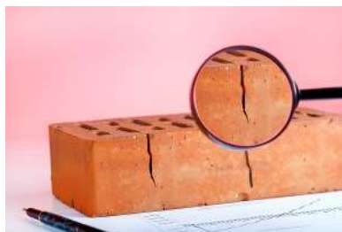
Figure 107: Defective Brick (Image Sergey Chuyko with permission)
