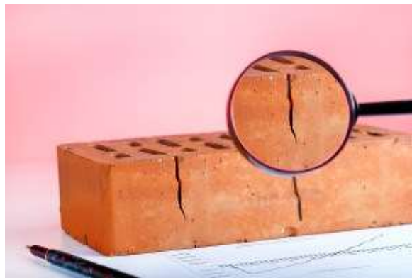
Figure 384: Defective brick (Image Sergey Chuyko with permission)
