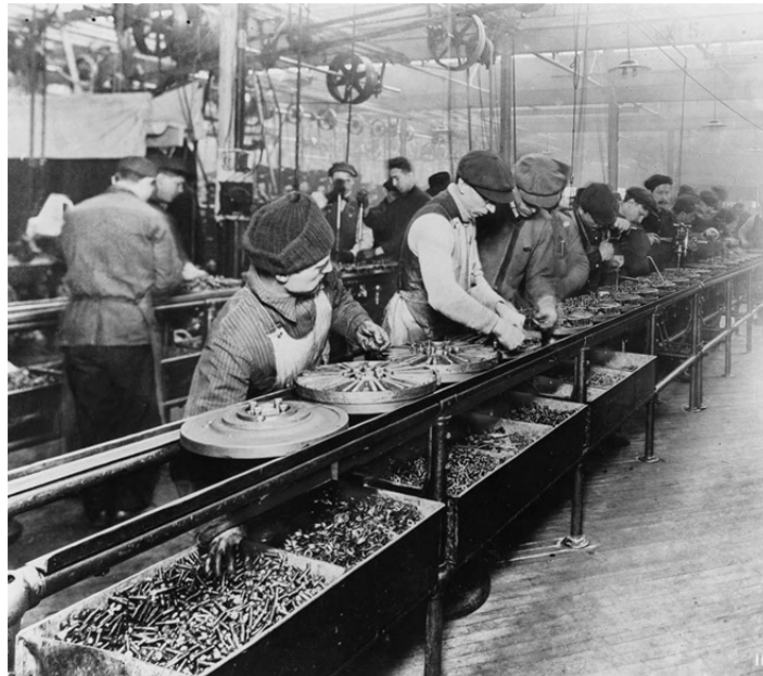
Figure 1: Ford Magneto assembly line, one of the first, if not the first, assembly line at Ford 1913 (public domain)
